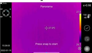
Users may enable the **panoramic stitching** function. In this function two or more images from the device are stitched into one panoramic. This function needs to be supported by ThermoAnalyze 3 software — **Image Stitching**.
