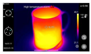
When the high-temperature alarm and low-temperature alarm switches are turned on at the same time, in order to ensure that the system is able to detect the set hightemperature alarm value, the low-temperature alarm value should not be higher than the high-temperature alarm setting.
