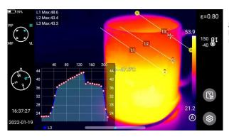
Up to 3 linear analysis objects can be added and displayed simultaneously in live mode.
