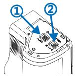
To install an SD card in the camera, unlock the security lid by sliding the latch on the compartment lid (1) and then open the lid by pulling the second latch (2).
