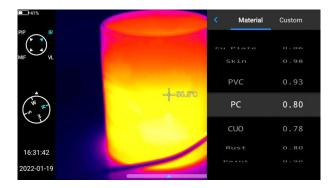
In the Real-time Image state, select the emissivity of the measured object by clicking the **Emissivity** bar. Press **Back** button or click any area on the screen other than the menu to return to the real-time interface. Then aim the center cursor at the measured object for temperature measurement.
