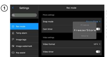
In the Real-time Image state, press the trigger button [5] to freeze the current scene, take images and save. Go to Settings ▶ Shoot mode and directly set the function of trigger button as image taking, thus achieving one-button taking pictures.
