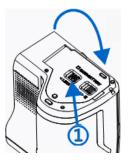
Close the lid and lock it with the latch (1). The card is now removed.
